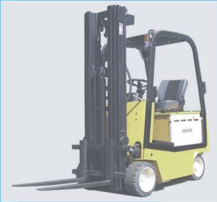
Electric Forklift with AC drive
