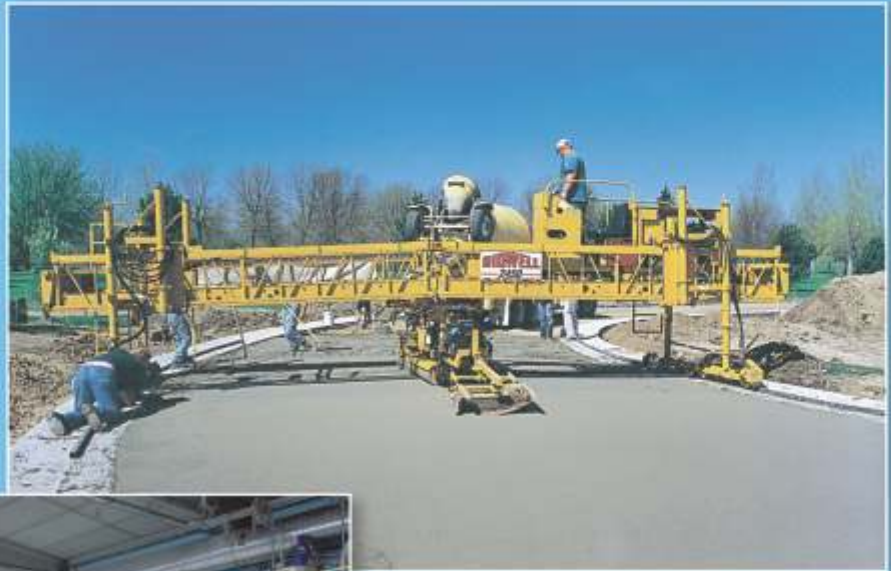
Bidwell 2450 Fixed Form Concrete Paver for highway construction
