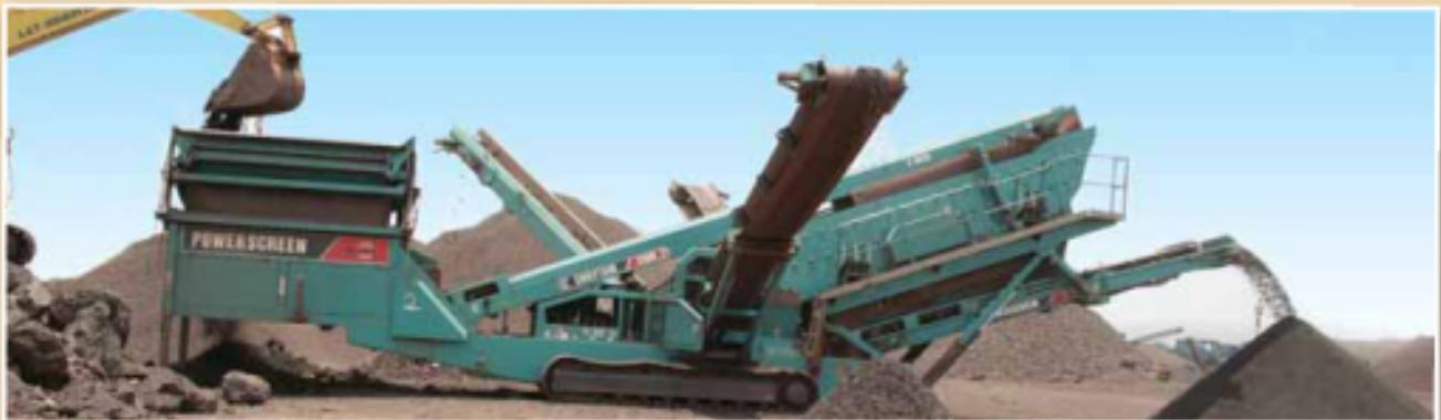
Powerscreen track mounted screening plant for mining and road construction
