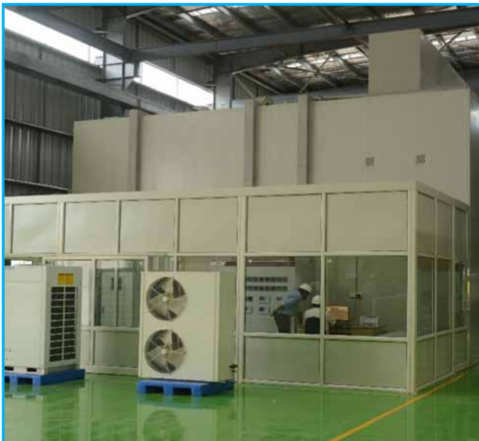
Multi-chambered Psychrometric Test Lab installed at the Voltas Waghodia Factory, one of the largest test facilities of its kind in India.
